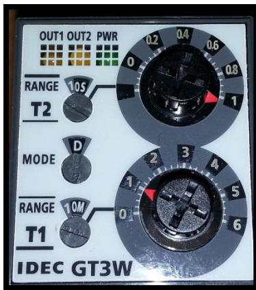
Figure 6 - Heatwheel defrost timer. The setting shown is the recommended setting for all Heatwheels.
