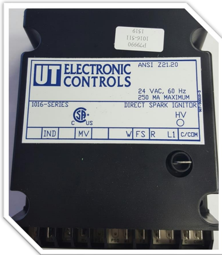
Figure 24 - Typical Ignition Control Module
